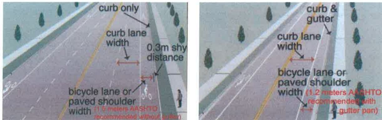
Figure 1: Curb lane width (CLW) measurements when there is no bicycle lane, no paved shoulder and no roadside parking. The left image shows a road with no gutter, for which CLW measurements require a 0.3-meter (1 foot) allowance, the space bicyclists typically leave between the bike and the curb. The right image shows a road with a gutter pan. CLW measurements in this case are made from the road/gutter seam to the center of the lane line.
